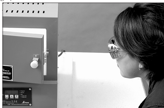
Crack the door open about 1/4" to check the progress of the glass or enameling. It takes only a couple of seconds.
