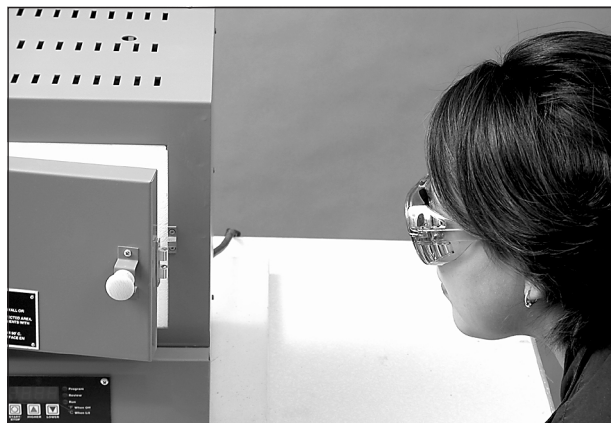
Looking at the glass during firing. Open the door about 1/2". Always wear green #3 firing safety glasses when looking at the hot glass.
