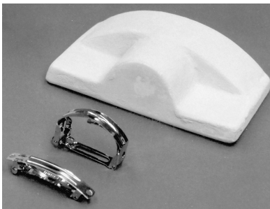
Shown is a hair barrette glass sagging mold. Sag the glass over the mold, and glue the glass to the barrette. Sagging molds are also available for glass bracelets.
